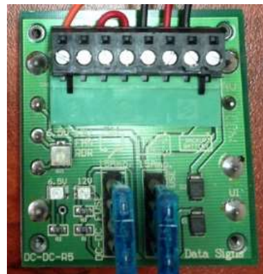
Controllers fitted with DC-DC converters, either external or internal
