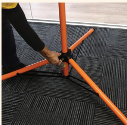
Step 5: Release the spring pin and ensure the tripod is locked.
