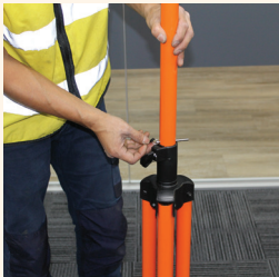
Step 3: Loosen locking tab, lift the post to the pin-hole & place pin.
