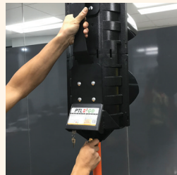
Step 9: Remove light from carry bag and fit onto stand. Pull spring pin and lower onto post. Release the pin into place.
