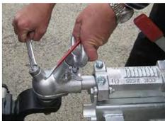
5. Tighten the locking nut firmly.
