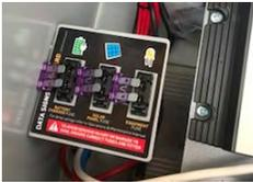
1. The power supply **MUST** be disconnected during manual lowering operation, pull out the **ALL** the fuses found under the shelf in the VSLs Control Box.
