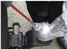
3. Using a flat-head screw driver on the slot on top of the pin, turn until tight, and then loosen very slightly. This will pull the coupling forward onto the tow ball and grip it.
