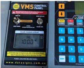
If the solar regulator does not appear to be on, check the SOLAR fuse is operational. The SOLAR FUSE can be found on the left of the solar regulator.
