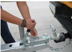
11. Release the hand brake if this is still engaged.
