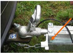
10. Ensure the Reversing lock on the tow coupling is released before travelling, as shown.
