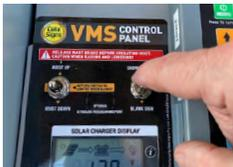
4. **Shutting Down: The sign MUST be BLANK when towed.**
