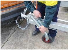
9. Wind up the jockey wheel and lift to slot into position. Make sure the jockey wheel does not move once in the towing position.
