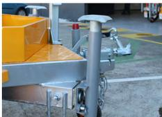
6. Pull the spring pin and rotate the wind-down legs upside down, ensuring the spring pin goes back in to lock the wind-down leg in the upwards position.
