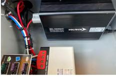
The Battery Charger is located under the shelf in the VSLS Control box.
