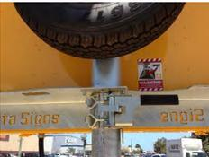
12. Feed the security chains through the wheels and fit the locks
