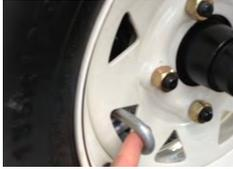
1. Remove the security chains from through the wheels.
