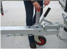
7. Use the Jockey wheel to lower the tow coupling onto the tow ball. Ensure the tow coupling fits snugly onto the tow ball of the towing vehicle. This is discussed further in this manual.
