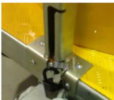
4. Slide lock-pin lever into bracket to hold and secure in place with a lock.
