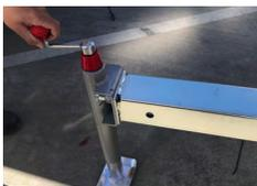
5. Retract the Wind down Legs up and slide in the outriggers on all four sides.
