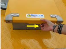
1. Raise the lid of the VSLS Control Box by sliding the concealed latch underneath the lid to the right.
