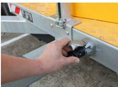
12. Plug the tow cable into the plug on the trailer and the towing vehicle. Check the trailer lights are functioning correctly.
