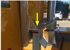
2. Undo the Mast Brake to lower the Sign Head.
