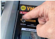
3. Lower the Sign Head using the Hoist Down switch on the VLSL Control Panel in the VLSL Control box.
